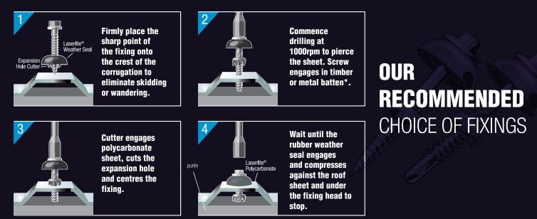
\*Always ensure the appropriate screw is being used for the batten you are drilling into.
