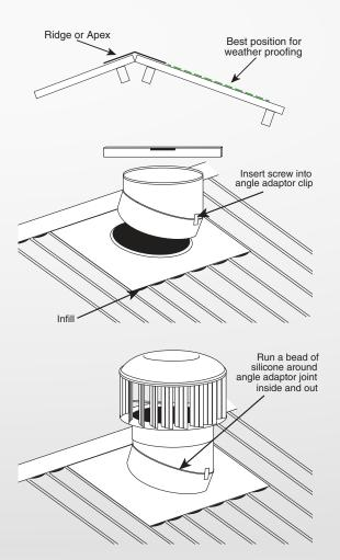
Either 10 gauge 16mm tek screw with neo or 4-3 blind rivets are recommended. When rivets are used apply silicone over the rivets to seal.
